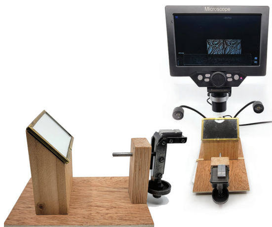
L: the base with angled mirror and type alignment gauge; R: base on the microscope for viewing type
