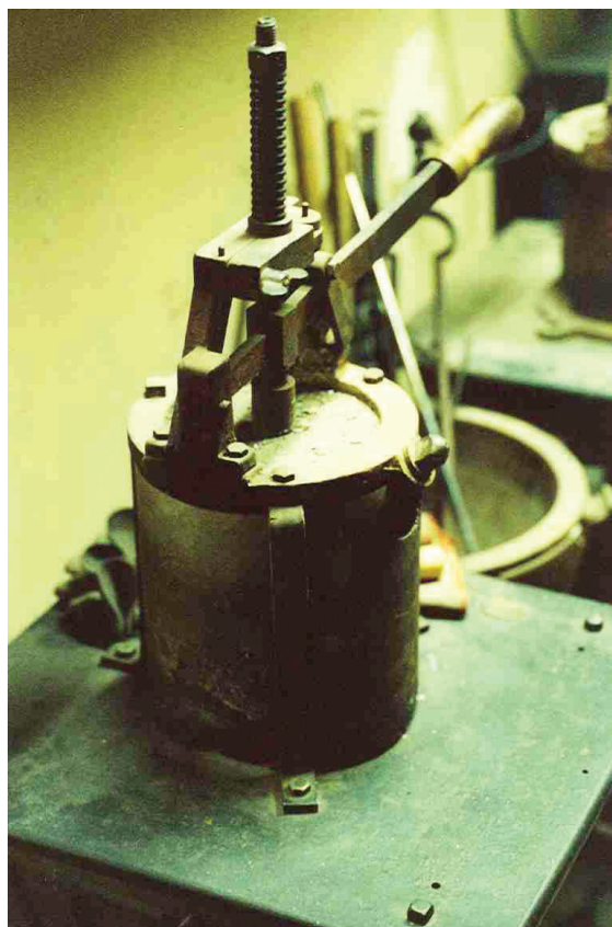
A force pump/pump pot. One of two that were in the collection of Theo Rehak. This one was sold to the Museum Plantin-Moretus to facilitate casting from their matrix collection. The second, barely seen in this photo, is in the workshop of Stan Nelson, Charles Town, WV.
